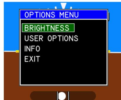
Pressing and holding the Control Knob for three (3) seconds will activate the User Options Menu. The manual brightness adjustment and info page are described in the IM. The Options Menu or User Options items will close and return to the active display after ten (10) seconds if no knob activity is recorded.
