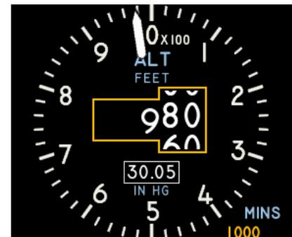
Once the MINS feature is active, turning the Control Knob left or right will change the minimum value. Once set, the MINS alert will activate when the aircraft descends past the set value after being above it. When activated, the border around the main altitude value (the 'counter drum window') will turn amber, along with the MINS numeric value. The alert will stay active until ascending 50 units above the minimum value or until the unit is power cycled.
