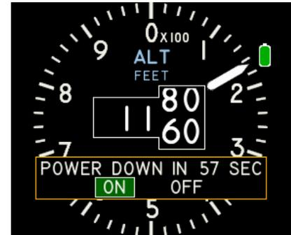
When this pop-up is displayed and you wish to power down the unit, either wait for the 60 second countdown to reach zero or turn the Control Knob to highlight the OFF option and press. This will send the Disable signal to the battery, thus removing power from the instrument.
