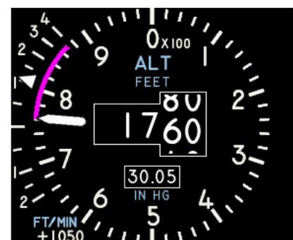
The VSI feature provides an analog scale from -2000 to +4000 feet per minute (or -10 to +20 meters per second) and a digital readout of the vertical speed up to  $\pm 9000$  feet per minute (or equivalent meters per second). The VSI units are determined by the configured altitude units (feet or meters).
