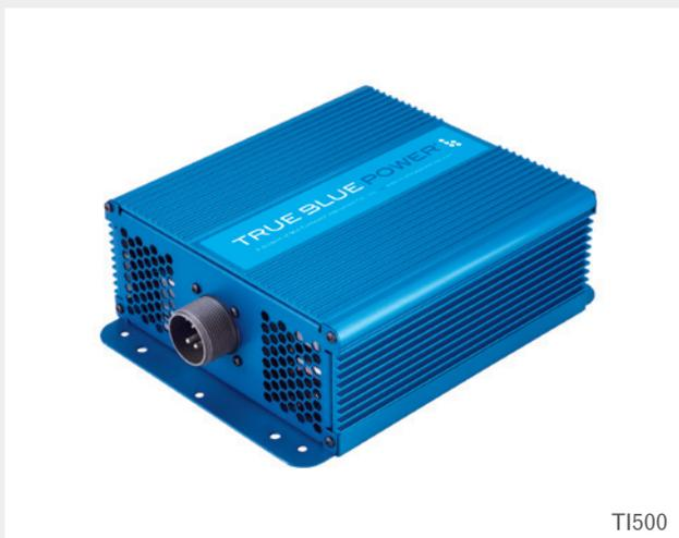
The TI500 DC-to-AC Inverter produces 115 volts at 60 Hz for 500 watts of “wall outlet” power from an aircraft’s 28 VDC input. Lighter and 30% smaller than competing inverters, the TI500 has the same connector and footprint of legacy designs, plus overload and short-circuit protection up to 150% of the rated load.
