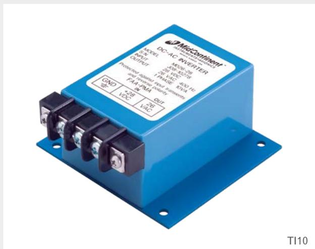
Standing just 1.5 inches tall, the TI10 DC-to-AC Inverter is a small, lightweight inverter designed to provide a reliable source of 26-volt, 400 Hz AC power. The voltage and frequency of its pure sine wave output remains stable regardless of input fluctuations.
